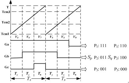
Figure 3 Alternative 3-segment switching sequence of sector
