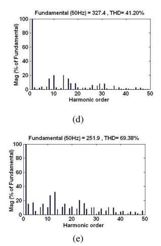
Figure 6 Harmonics spectrum of 3-segment SVM
