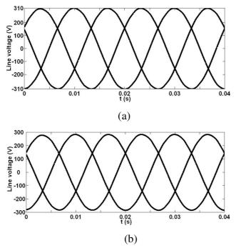
Figure 4 Output line voltage when  $m \le 1$
