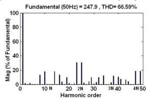
Figure 7 Harmonics spectrum of 7-segment SVM with N = 12
