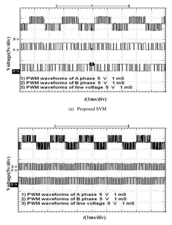
(b) 7-segment SVM Figure 10 PWM waveforms
