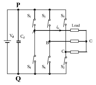
Figure 1 Three-phase inverter
