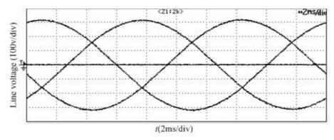
Figure 8 Proposed SVM test waveforms of line voltage with m = 1
