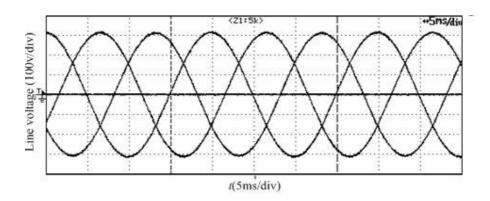
Figure 9 7-segment SVM test waveforms of line voltage with m = 1
