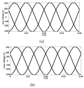
Figure 5 Output line voltage in overmodulation region
