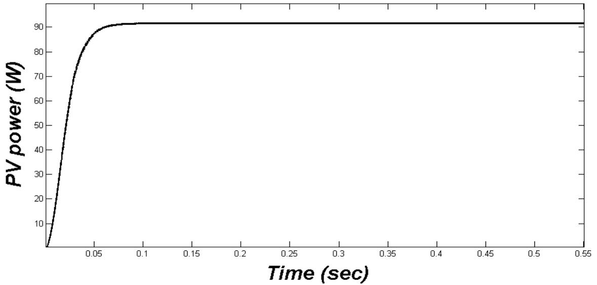
Fig. 10. Output Power of PV
