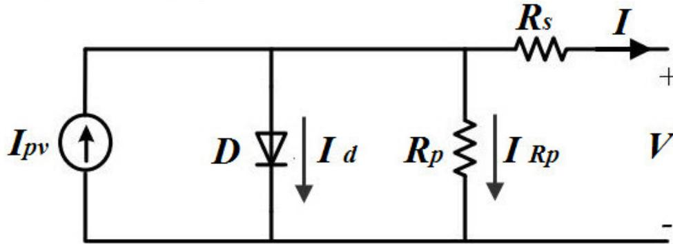
Fig. 1. Equivalent circuit of one photovoltaic array
