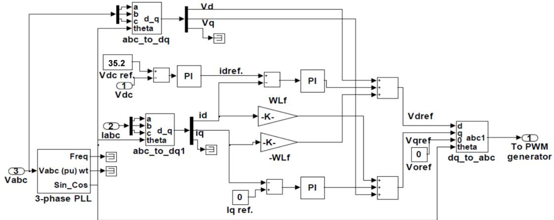
Fig. 8. The inverter control model
