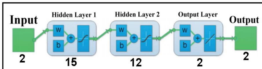
Fig. 2. Feed forward neural network for MPPT
