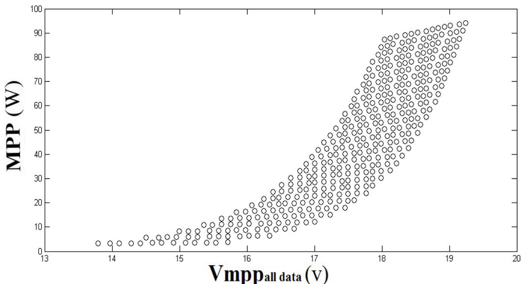
Fig. 5. The output of  $V_{mpp}$  -  $M_{pp}$  optimized by (GA)
