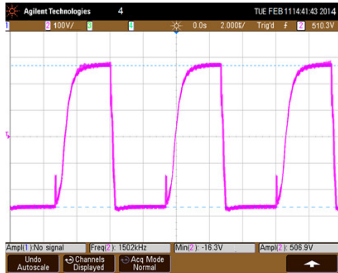
Figure 11. Experimental Output voltage waveform tested at 500V source resistance of 25Ω.
