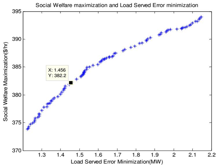
Figure 1: Pareto optimal front of SWM and LSE minimization with voltage dependent load modeling using SPEA 2+.
