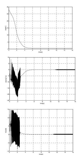
Figure 8 : Angle, velocity and force for initial angle equal to 28°
