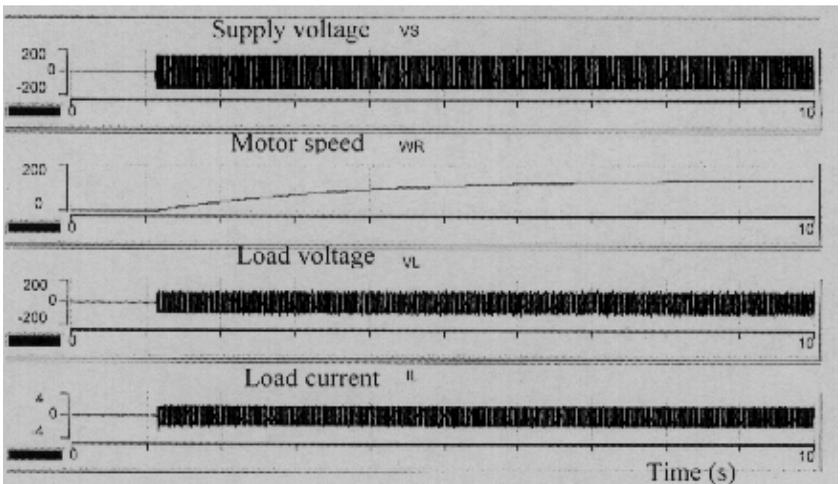
Fig. 9 Open loop run-up behavior for half load
