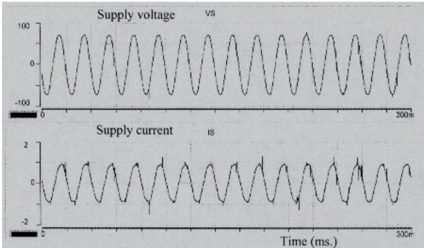
Fig. 3 Experimental waveforms for supply voltage and current.
