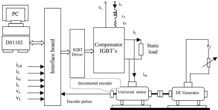
Fig. 2 Experimental set-up for DSP-based control
