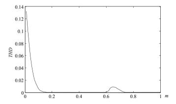
Fig. 12: Load voltage THD for different modulation indexes.
