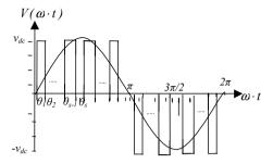
Fig. 2: Output Voltage Waveform of a three-level inverter angle SHE-PWM.
