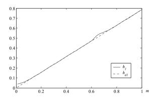
Fig. 10: Fundamental load voltage ( $h_1$ ) versus modulation index (m) in a two-level three phase inverter with the proposed modulation scheme.
