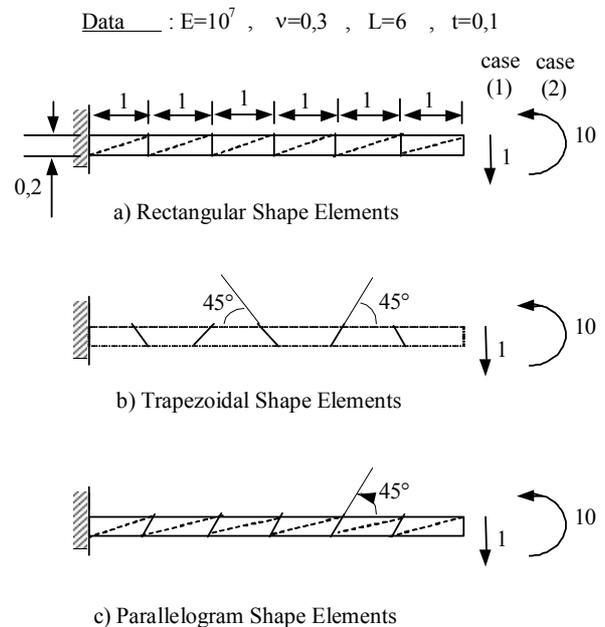
Fig.14 : MacNeal's elongated beam. Data and mesh.
