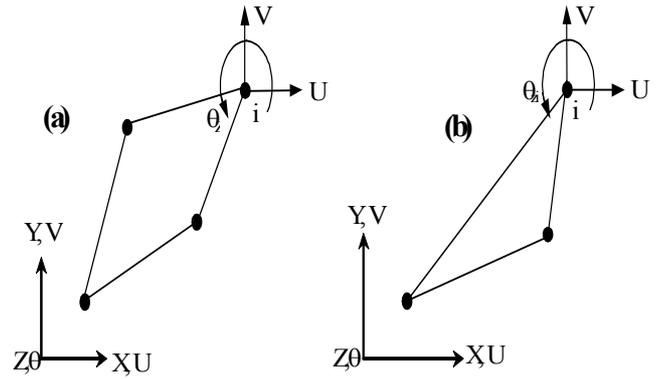
Fig 1 : Quadrilateral and triangular elements
