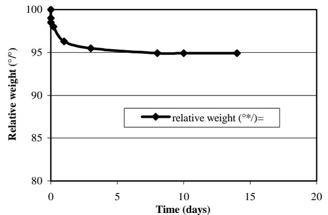
**Figure 1 : Methanol exchange of cement paste, w/c=0.4 65 days old**
