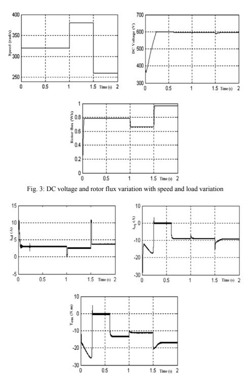
Fig. 4: Dynamics of the SEIG during startup and load variation at 0.6 s
