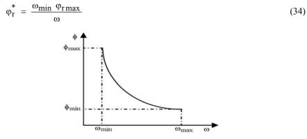
Fig. 2: Relationship between rotor speed and rotor flux linkage.
