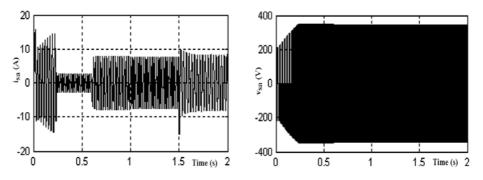
Fig. 5: Generated current and voltage at the terminals of induction generator with load variation at 0.6 s
