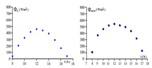
Fig. 6: Solar flux density received by the concentrator, solar rays normal to aperture
