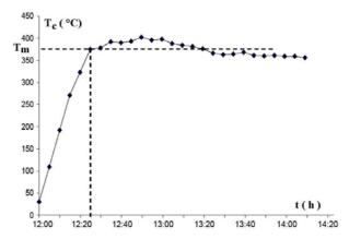
Fig. 8: Temperature profile of the disk center
