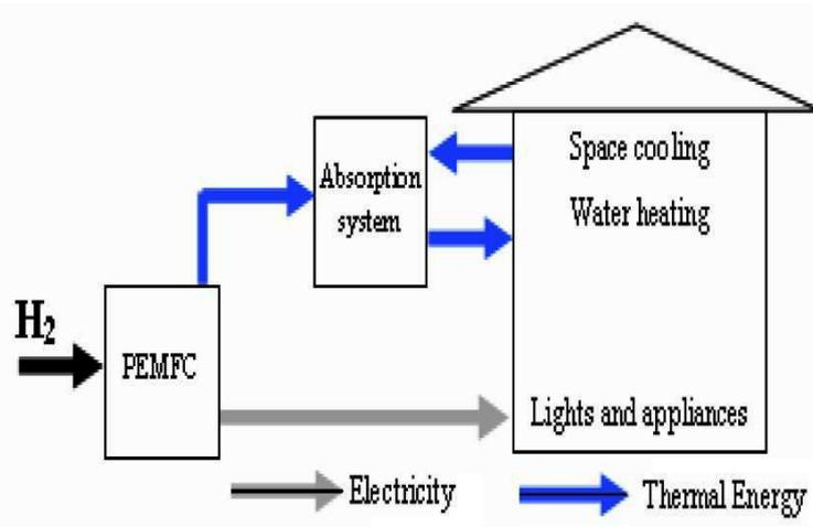
Fig. 1: Schematic description of the PEMFC energy system
