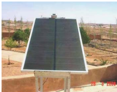
Fig. 1: PV module type US 645 in outdoor exposure
