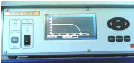
Fig. 2: Representation of experimental set up based on data acquisition PVPM 2540C
