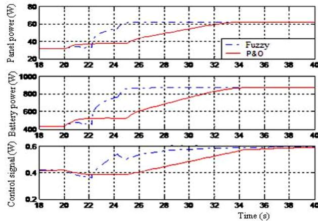
Fig. 11: Fuzzy and P&O controller responses: for a fast solar insolation increase (500 W/m<sup>2</sup> to 1000 W/m<sup>2</sup> in 5 s at 25 °C)
