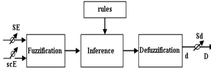
Fig. 7: General diagram of a fuzzy controller
