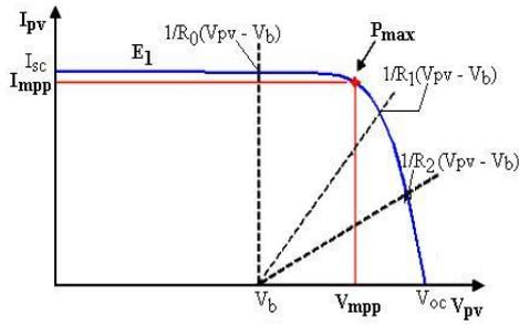
Fig. 1: Current-voltage characteristic of a PV module
