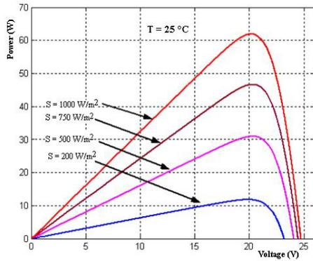
Fig. 4: Influence of the solar radiation for constant temperature
