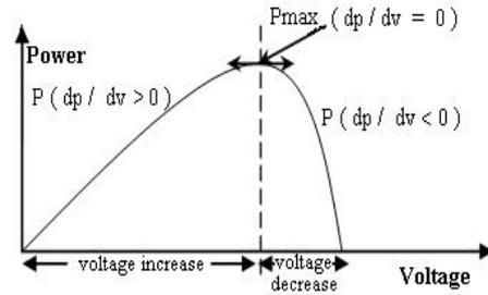
Fig. 2: Power-voltage characteristic of a PV module
