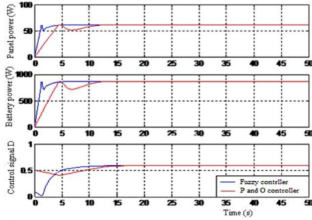
Fig. 9: Variation of the panel power, battery power and the duty ratio D, under standard conditions: temperature (25 °C) and solar insolation (1000 W/m<sup>2</sup>)
