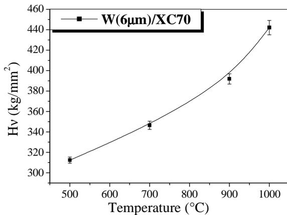
Fig. 3: Variation of the micro-hardness in function of the temperature of annealing.
