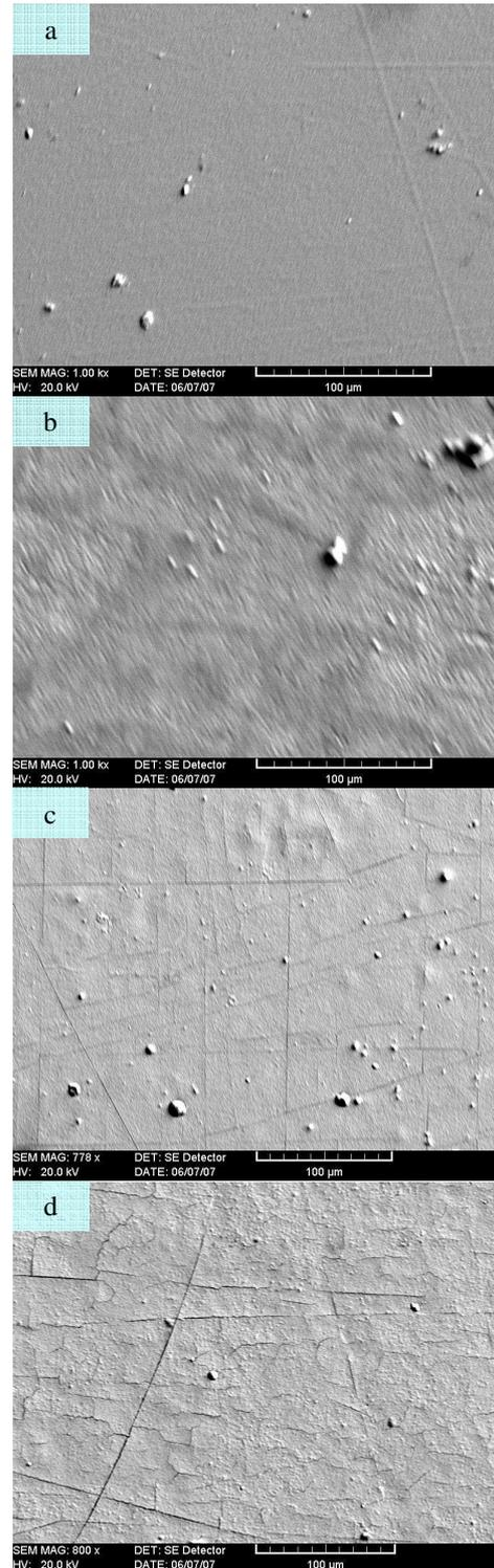
Fig.2: SEM surface images of the samples [W (6µm)/XC70]: before (a) and after annealed during 30 min at  $700^\circ\text{C}$  (b),  $900^\circ\text{C}$  (c) and  $1000^\circ\text{C}$  (d).
