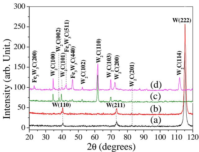
Fig. 1: XRD spectra of the samples [W (6µm)/XC70]: before (a) and after annealed during 30 min at  $700^\circ\text{C}$  (b),  $900^\circ\text{C}$  (c) and  $1000^\circ\text{C}$  (d).
