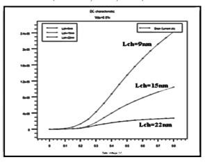
Figure 7. Transfer characteristics for a dual metal gate GAA MOSFETs at different channel length (Lch-9nm, 15nm, 22nm).
