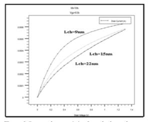
Figure.6 Output characteristics for a dual metal gate GAA MOSFETs at different channel length (Lch=9nm, 15nm, 22nm).
