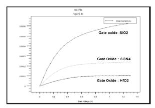
Figure..8 Output characteristics for a dual metal gate GAA MOSFETs at different High-k dielectric type (SiO2, Si3N4 and HFO2).
