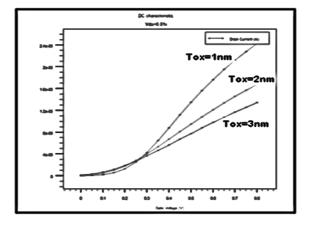
Figure.5 Transfer characteristics for a dual metal gate GAA MOSFETs at different oxide thickness (Tox=1nm, 2nm, 3nm).
