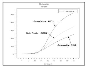
Figure. 9. Transfer characteristics for a dual metal gate GAA MOSFETs at different type of oxide (SiO2, Si3N4 and HFO2).
