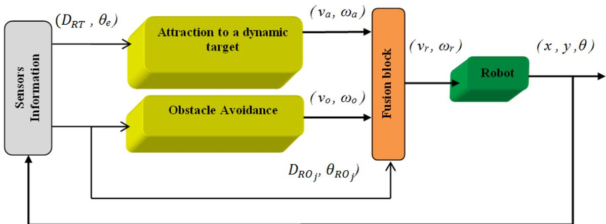
**Fig. 5.** The proposed control scheme.
