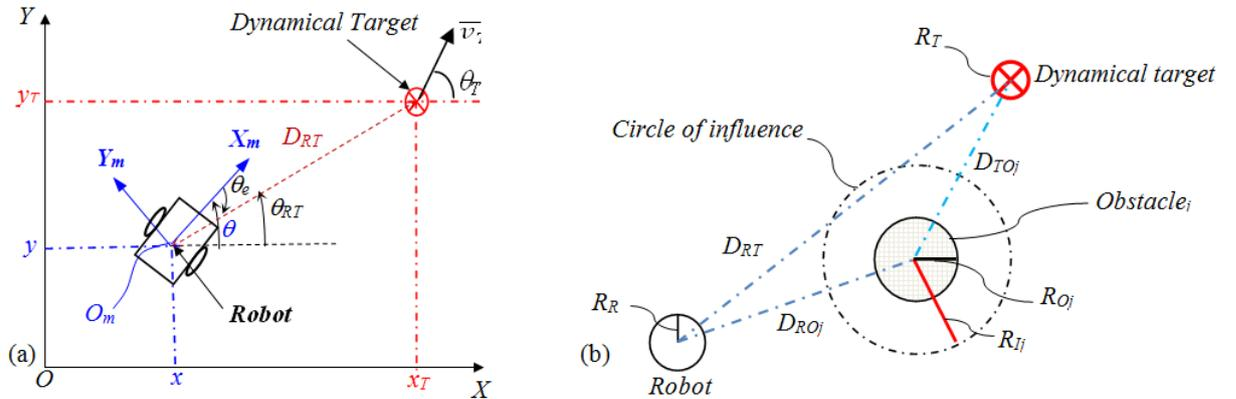
**Fig. 1.** (a) Attraction to a dynamic target and (b) The used perceptions for mobile robot.
