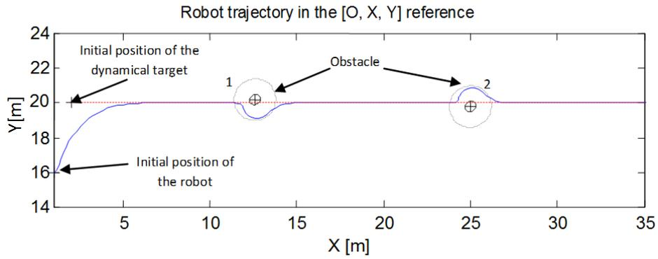
**Fig. 6.** Robot trajectory reaching a dynamic target (moving straight) while avoiding obstacles.
